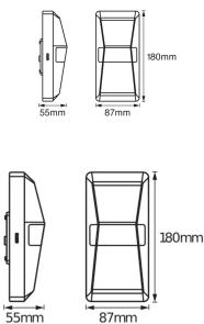
**Specifications Ledvance Endura Pro Wall Light White Up & Down - 10W 1000lm - 840 Cool White | IP55 - Motion and Light Sensor**
